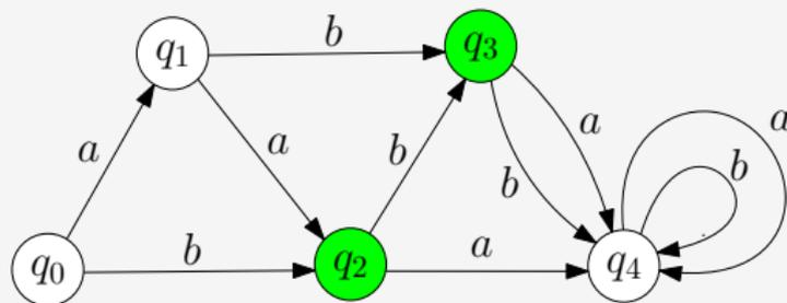
Figure: A DFA. This is the minimal DFA recognising the language  $\{aa, aab, ab, b, bb\}$ .
